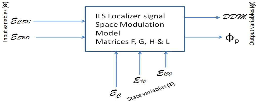
**Fig. 3.3. Concept of ILS localizer signal modeling**
