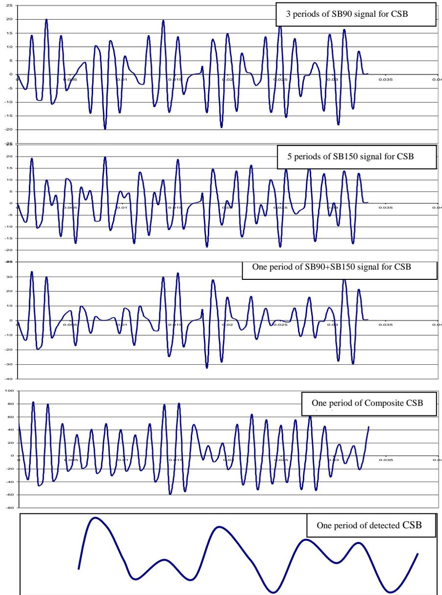
**Fig. 2.6. Generation, processing and detection of CSB signal**
