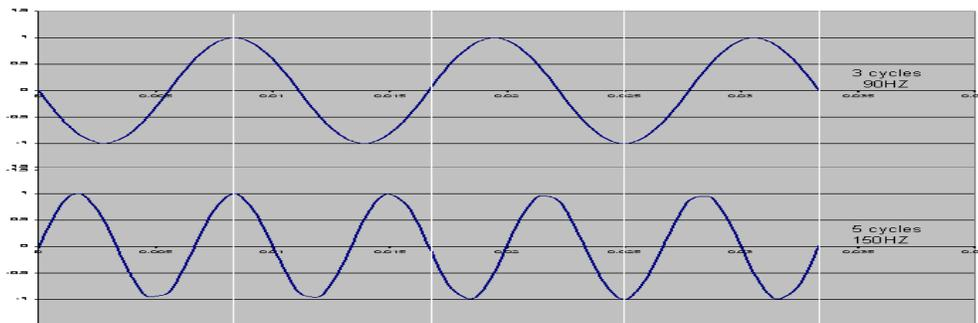
**Fig.2.5. 90HZ and 150HZ in PHASE-OPPOSITION for the SBO signal**
