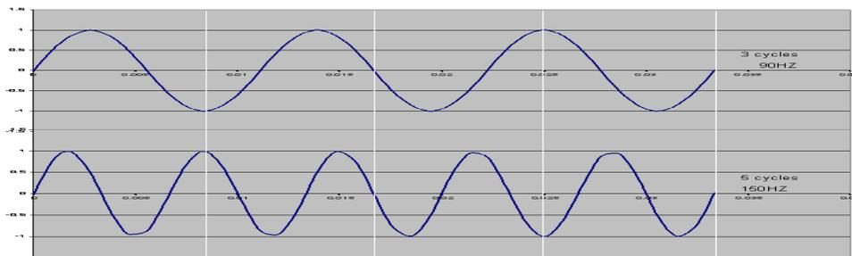
**Fig.2.4. 90HZ and 150HZ IN-PHASE for CSB signal per definition**
