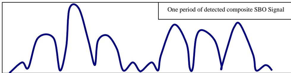
**Fig.2.8. One Period of detected composite SBO signal**
