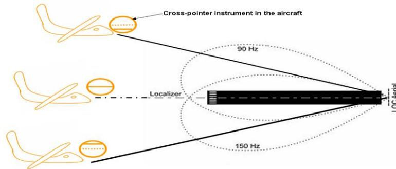
**Fig.2.1. Principle of the ILS Localizer**
