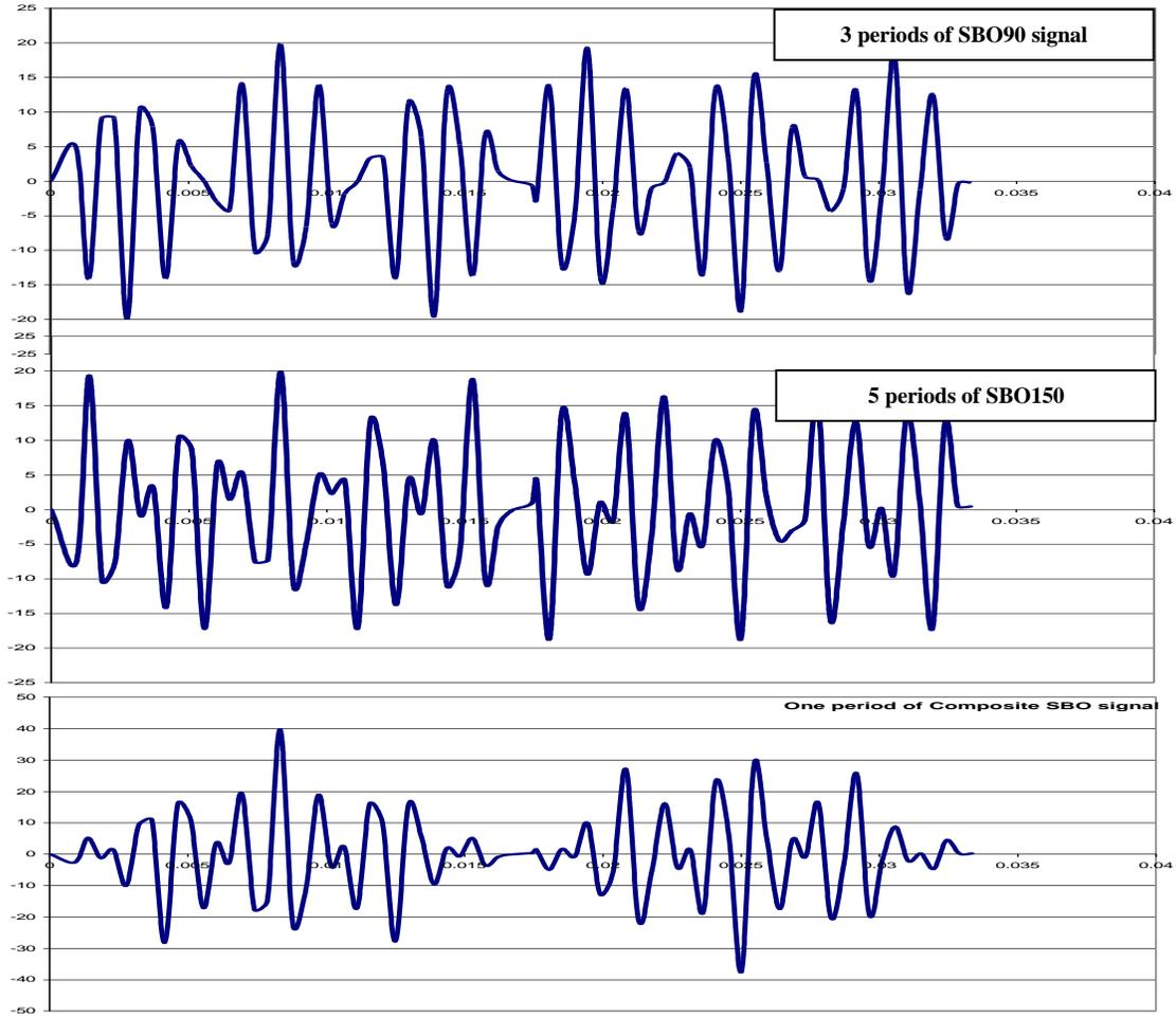
**Fig. 2.7. Generation of SBO signal**
